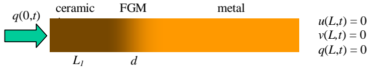
Figure 1. Schematic representation of the FGM bar lay-up and dimensions
