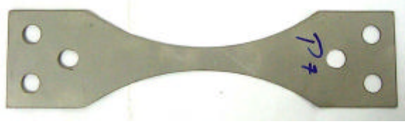
Figure 2. Smooth specimen used in this research. Length = 200 mm; Width = 12.7 mm.
