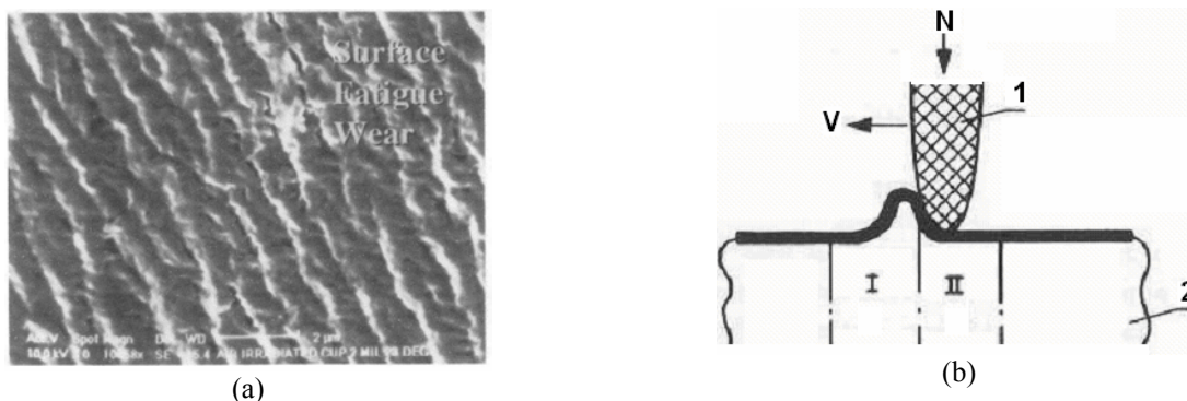
Figura 1– (a) SEM micrographic of UHMWPE, surface of total joint replacement (Wang et al. , 1998), (b) Illustration of the wear mechanism that leads to the wave-like formation: (I) compression zone, (II) stretching zone (Bartenev and Lavrentev, 1981).
