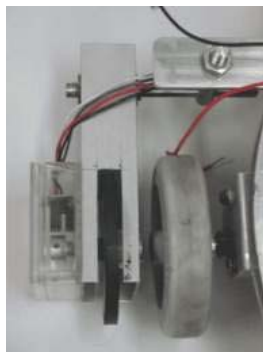
Figure 5 - Physical mounting of one of the encoders used in ROMEO III.
