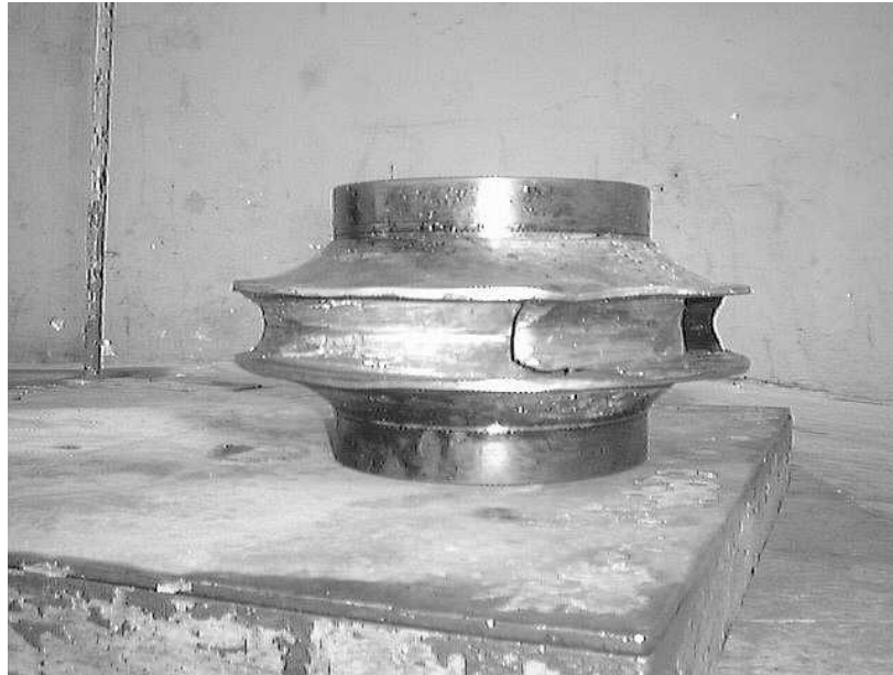
Figure 3. Impeller of the damaged pump
