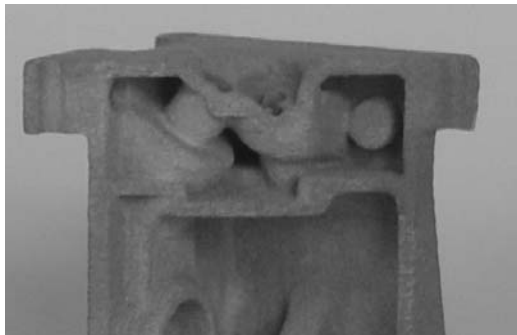
Figure 4 - Second head design, with water jacket
