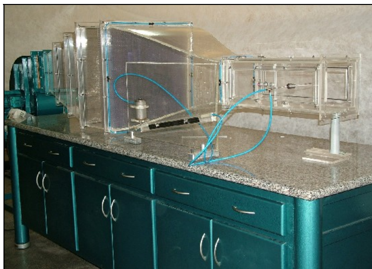
Figure 1. Aerodynamic Tunnel of the Flow Visualization Laboratory
