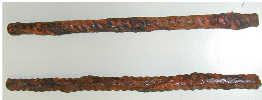
Figure 7 - Specimens after 2016 hours of exposition in the corrosion chamber.
