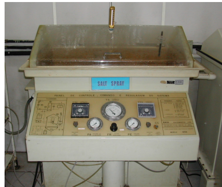
Figure 6. Corrosion Chamber for Salt Spray Test.
