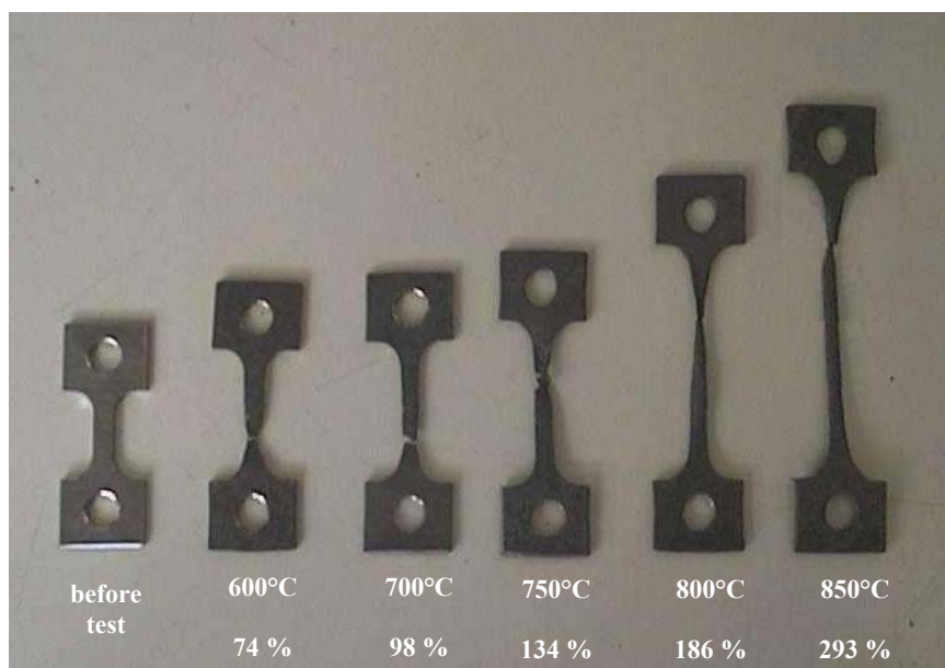
Figure 13 – Tensile specimens having different elongation until rupture at different temperatures and same crosshead speed V_c = 0.05 mm/min.
