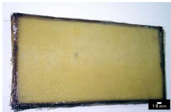
Figure 2 - Composite plate after cure for 24 hours at room temperature.
