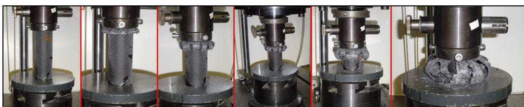
Figure 10. Evolution of failure in a quasi-static test
