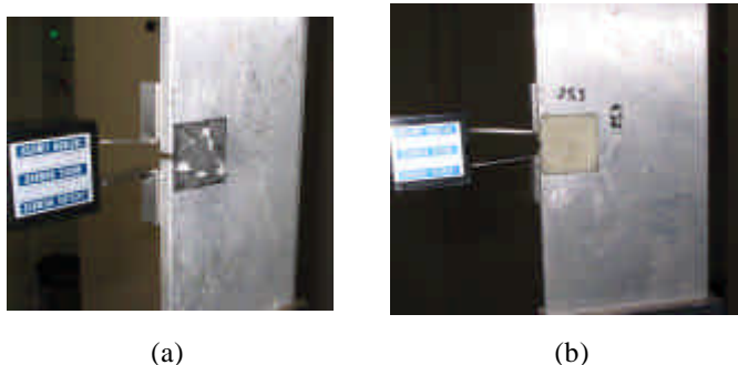
Figure 3 - Patch bonded to the specimen on one of its surface: (a) carbon fiber and (b) glass fiber
