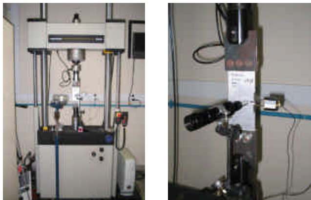
Figure 2 - INSTRON Model 8802 and specimen assembly with COD GAGE and lunette 80x
