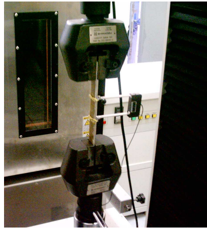
Figure 5. Specimen with extensometer mounted.
