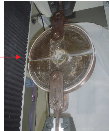
Figure 5. Hoop tensile strength test with a split-disk device.
