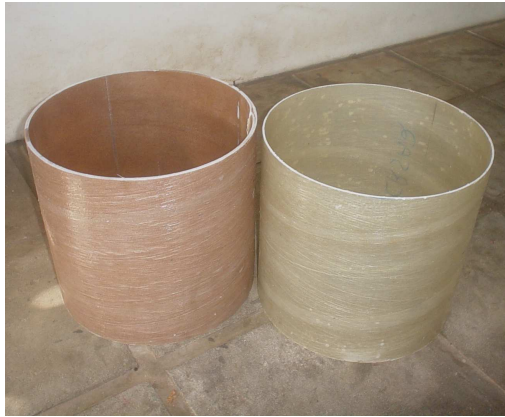
Figure 6. Parallel-plate loading stiffness test samples.
