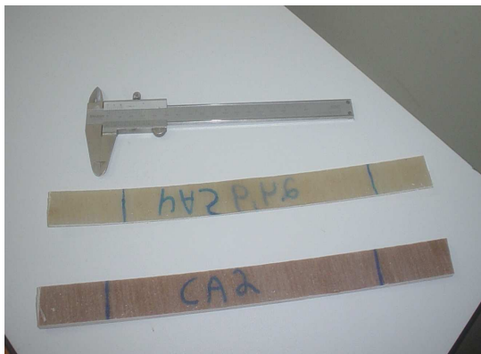
Figure 2. Longitudinal tensile strength test samples.
