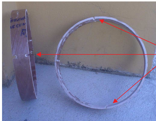
Figure 4. Hoop tensile strength test samples.
