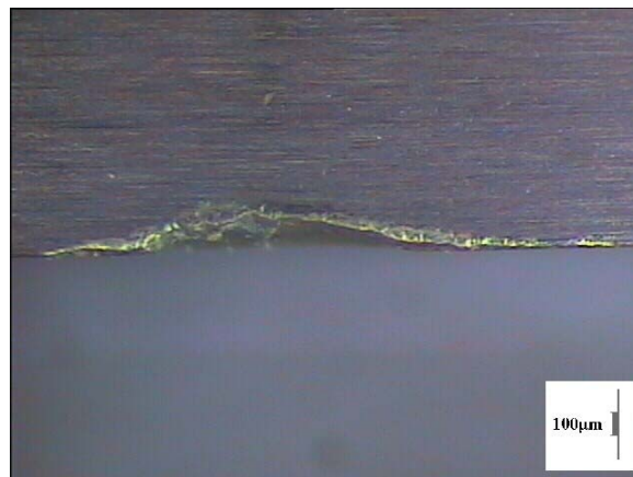
Figure 6 – Cutting edge in the end of the experiment with b = 8 , n = 3,000 RPM
