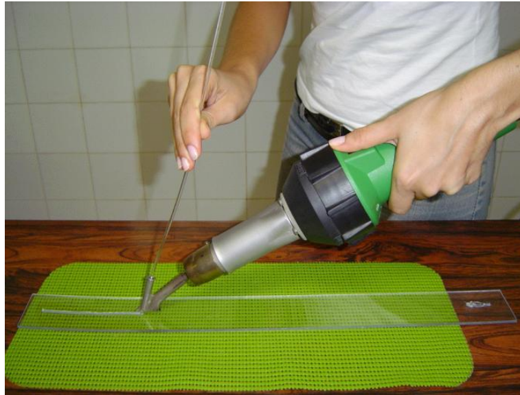
Figure 1. Bead-on-plate welding on a PC plate
