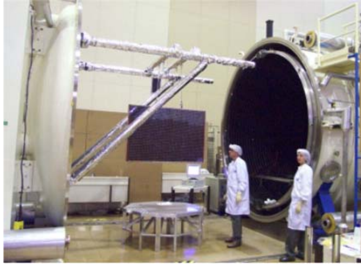
Figure 5: T2-P1-CP1 Test Specimen being prepared for the thermal vacuum test at LIT/INPE.
