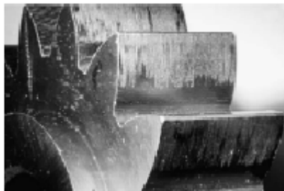
Figure 7. FZG Gear standard scuffing (Höhn, 2004)
