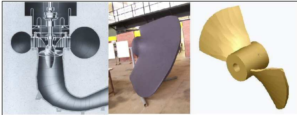
Figure 1: Reverse engineering for building a CAD model of a turbine rotor - GRACO/UnB. In the left, a vertical section of a Kaplan turbine. To the center, a single-blade turbine mockup. To the right, the computer model of the turbine rotor obtained from a contact profile digitizer.
