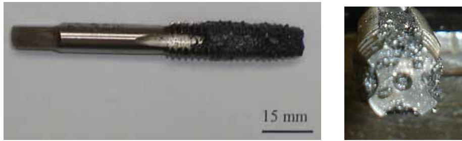
Figure 6. Illustrative photos of a tap tool after machine grey cast iron under lubricated conditions (MQF).
