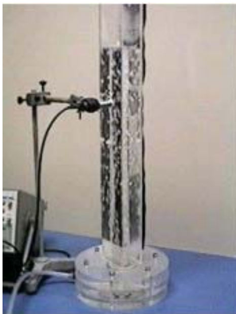
Figure 1. Column with bubble flow in liquid medium
