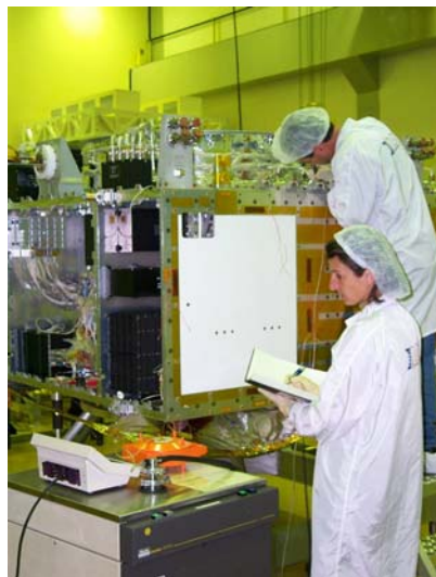
Figure 4. Local Leak Tests - INPE
