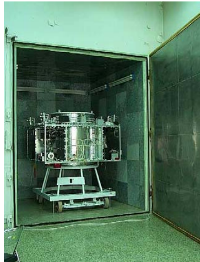
Figure 7. CBERS FM2 in Atmospheric Chamber for the Global Leak Tests procedures - China
