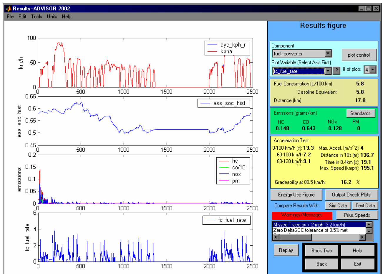
Figure 1. Results from ADVISOR for simulation of Vectra Hybrid with ICE 1.9 and EM with 49kW. Graphics curves represent model speed against cycle demand, SOC of battery pack, emissions produced over driving cycle and fuel consumption rate by ICE. Data in right side shows final values for the simulation.
