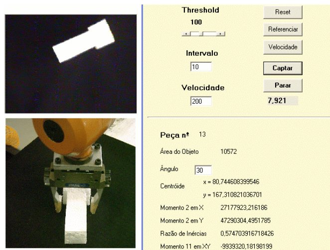
Figure 4. Capture screen, processing module and manipulator picking an object
