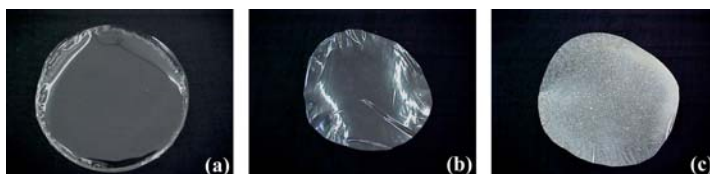
Figure 1. Dense chitosan membranes visual aspect: (a) formulation 1, (b) formulation 2, (c) formulation 3.
