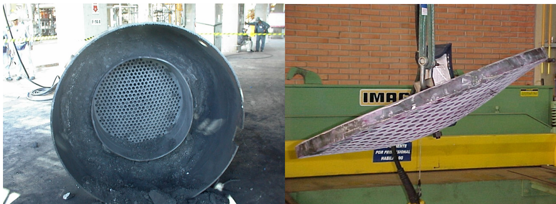
Figure 2. (a) Aspect of the liner after failure. (b) Deformed perforated plate
