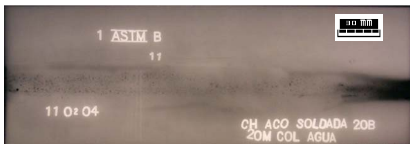
Figure 6 – Weld bead radiograph made at 20 meters depth
