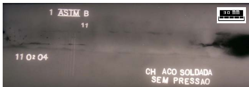
Figure 5 – Weld bead radiograph made at zero meter depth
