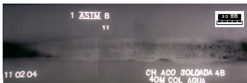
Figure 7 – Weld bead radiograph made at 40 meters depth
