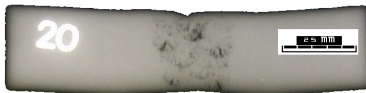
Figure 10 –Radiograph of cross-section sample removed from welded joint made at 20 meters depth
