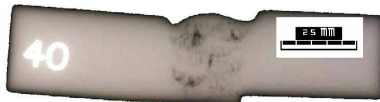
Figure 11 –Radiograph of cross-section sample removed from welded joint made at 40 meters depth
