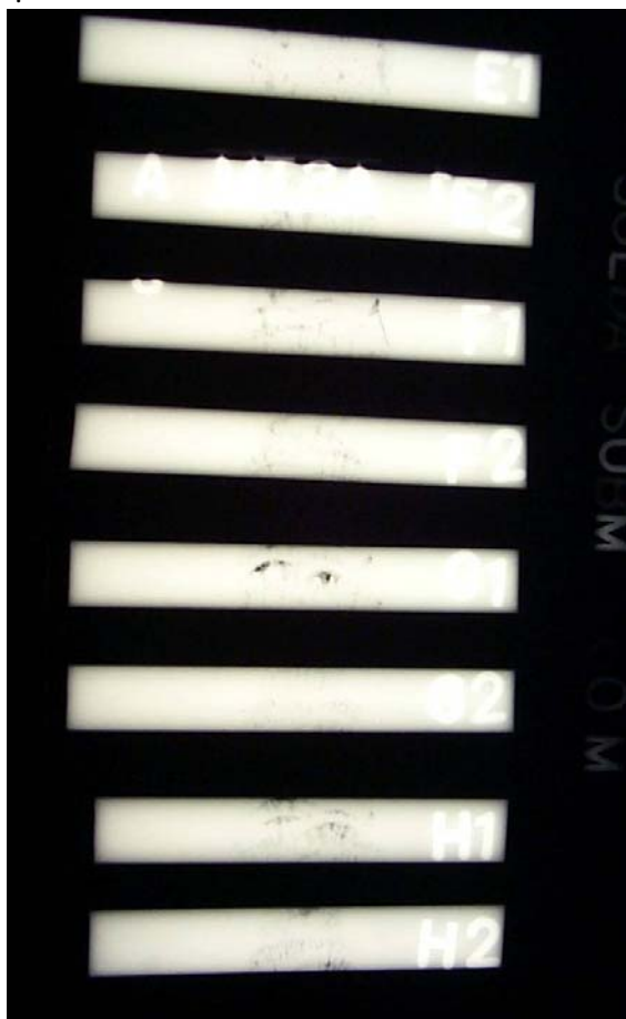
Figure 13 – Radiographs taken of 0° of Charpy pre-machined samples removed from welded joint made at 60 meters depth
