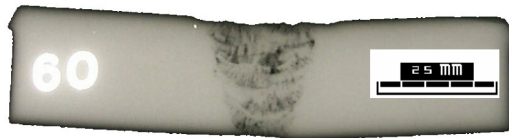
Figure 12 –Radiograph of cross-section sample removed from welded joint made at 60 meters depth
