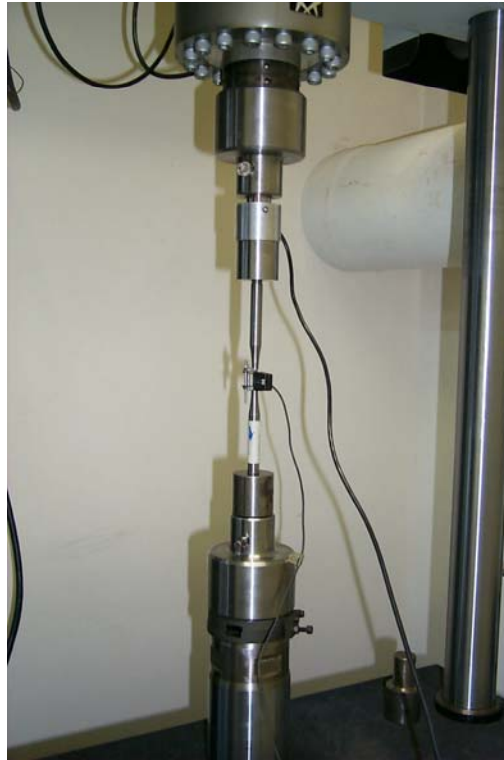
Figure 1. Experimental set-up used for the axial fatigue testing of the AISI 8620 steel specimens..
