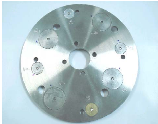
Figure 2. Rotating disk and the test specimens.
