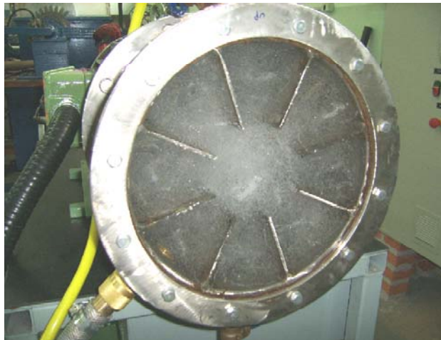
Figure 1. Cavitation test chamber
