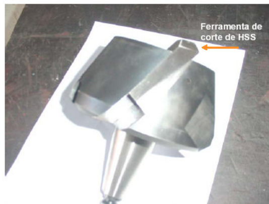
Fig 3- Cabeçote porta ferramenta conforme norma Volvo (The Volvo Standard Machinability Test, “Std. 1018.712”, 1998).
