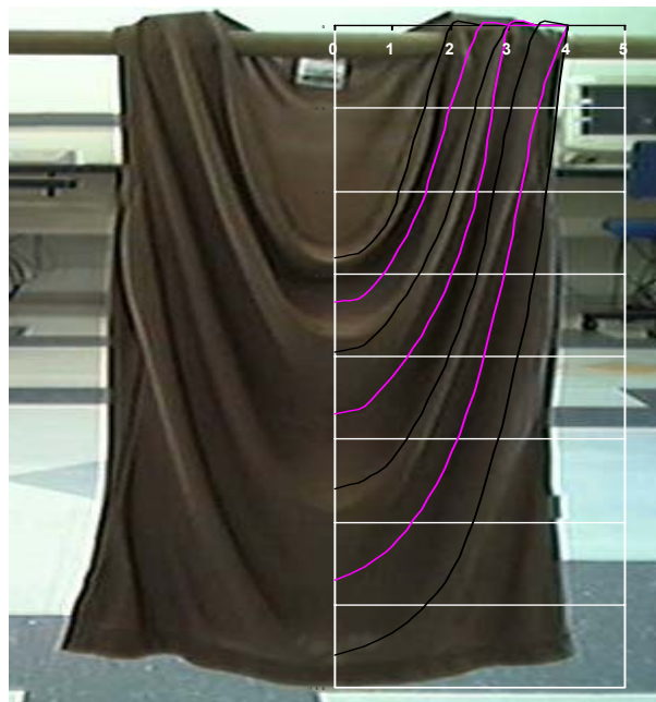
Fig. 7 - Folds obtained by the approach drawn over a real shirt (red lines represent negative folds)
