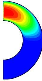
Figure 4. Isolines of turbulent kinetic energy for  $Ra^*=2.0 \times 10^2$  and  $R=2$ .
