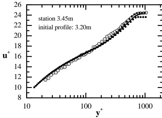
Figure 6: Calculated downstream velocity profiles using experimental and estimated initial profiles; inner variables. Points denote experiments; filled squares, initial profile given by inverse method; filled circles, initial profile given by classical approach; line, initial profile given by experiments.
