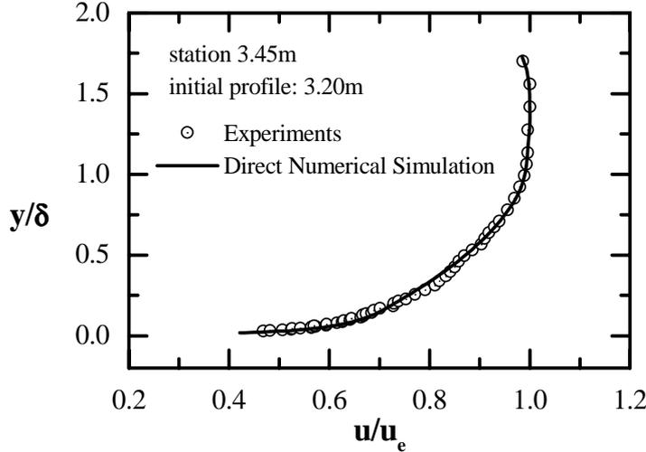
Figure 1: Validation of the numerical solution for the direct problem. Comparison of calculated and measured velocity profiles. Points denote the experimental data.
