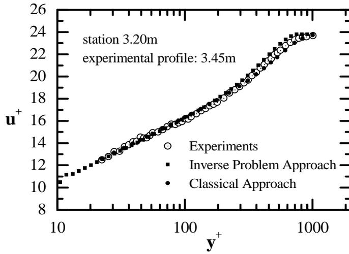
Figure 4: Comparison of estimated initial velocity profile in inner variable with experimental data using one measured at station 3.45m.
