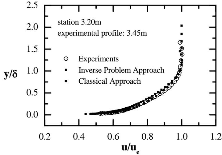
Figure 3: Comparison of estimated initial velocity profile with experimental data using one measured velocity profile at station 3.45m.
