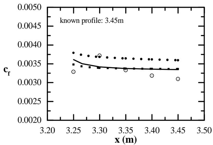
Figure 7: Estimation of friction coefficient using one measured station, 3.45m. Points denote experiments; filled squares, inverse method; filled circles, classical approach; line, direct method.
