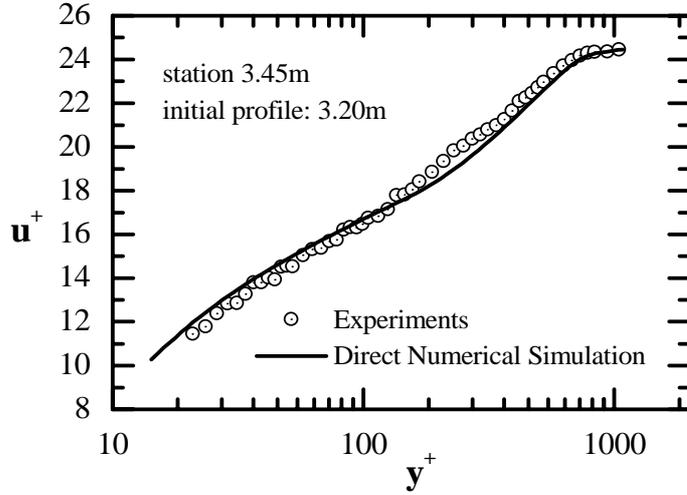
Figure 2: Validation of the numerical solution for the direct problem. Comparison of calculated and measured velocity profiles in inner variable.
