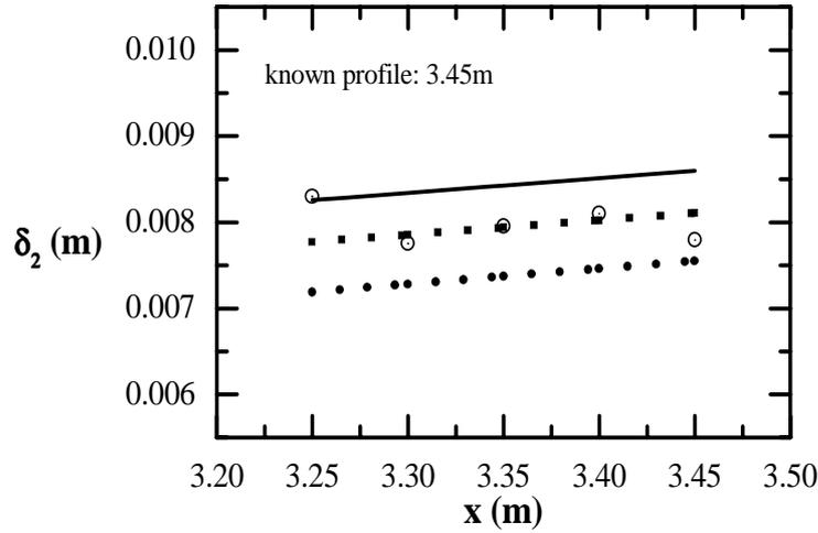
Figure 8: Estimation of momentum thickness using one measured station, 3.45m. Points denote experiments; filled squares, inverse method; filled circles, classical approach; line, direct method.
