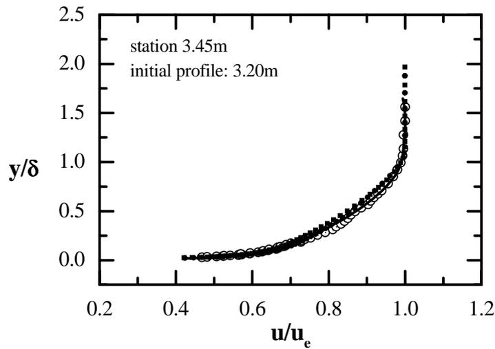
Figure 5: Calculated downstream velocity profiles using experimental and estimated initial profiles. Points denote experiments; filled squares, initial profile given by inverse method; filled circles, initial profile given by classical approach; line, initial profile given by experiments.
