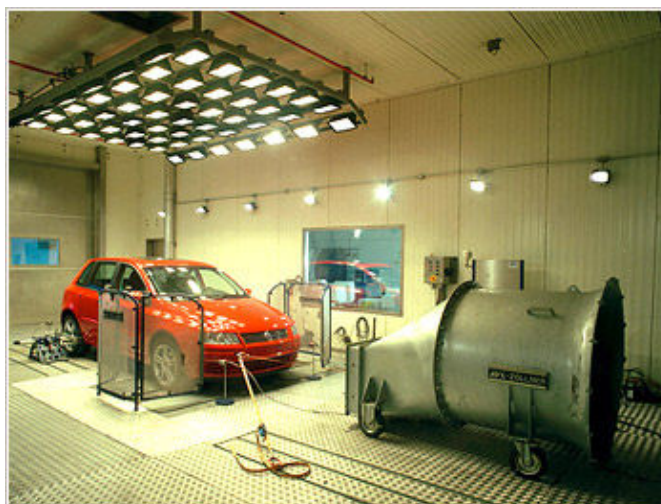
Figure 8. Climate chamber with roller dynamometer.
