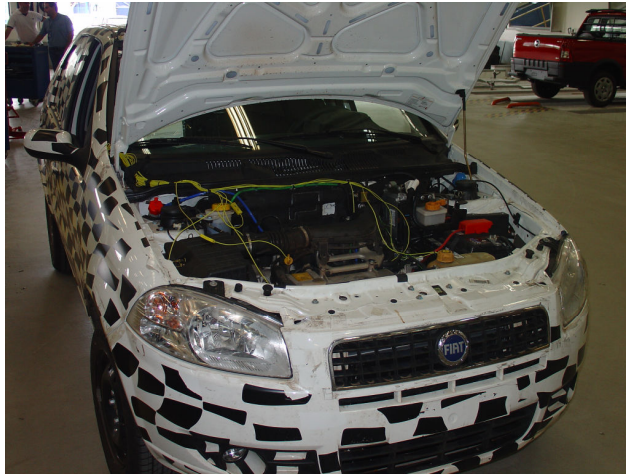
Figure 9. Instrumented vehicle to ATB test.
