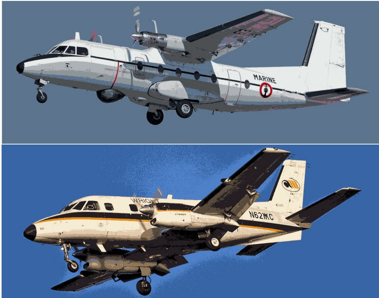
Fig. 25 – Bandeirante EMB 110 (bottom) and its inspiration (top), the Nord 262 airliner. The 29-seater Nord 262 high-wing monoplane is derived from the MH250 Super Broussard, which was designed by Max Holste.
