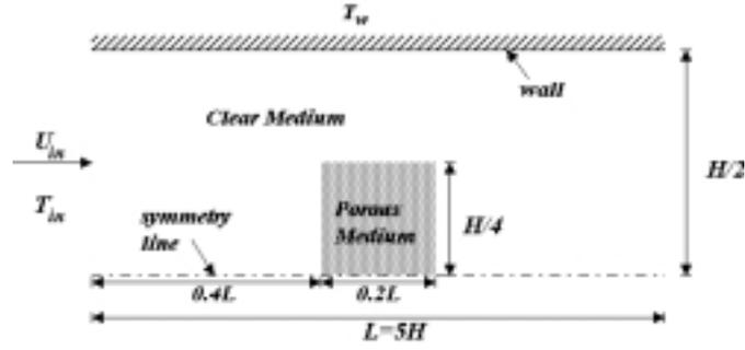
Figure 2 - Problem geometry and dimensions.
