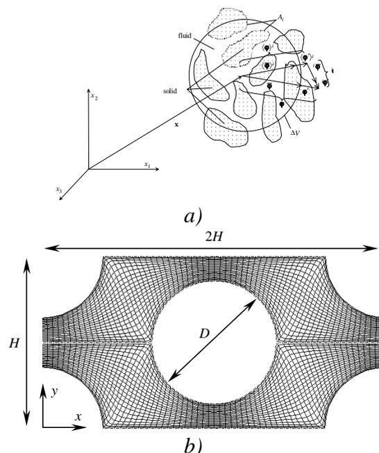
**Figure 1 – a) Representative Elementary Volume (R.E.V.), b) Model of R.E.V, periodic cell and non-orthogonal grid.**
