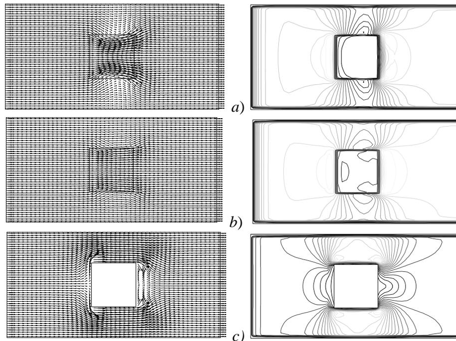
**Figure 4:** Taken from de Lemos & Pedras, 2000b. Two-dimensional maps for  $\bar{u}_D$  (top) and  $\langle k \rangle$  (bottom). Turbulent flow:  $Re_K = 3.5 \times 10^3$ ,  $K_2 = 2.34 \times 10^{-4}$  and  $\phi_1 = 0.40$ : a)  $\phi_2 = 1.0$ , b)  $\phi_2 = 0.8$  and c) solid obstacle.
