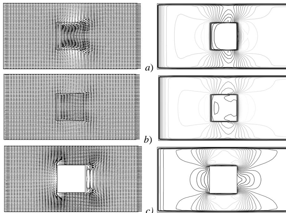
**Figure 4:** Taken from de Lemos & Pedras, 2000b. Two-dimensional maps for  $\bar{u}_D$  (top) and  $\langle k \rangle^i$  (bottom). Turbulent flow:  $Re_K = 3.5 \times 10^3$ ,  $K_2 = 2.34 \times 10^{-4}$  and  $\phi_1 = 0.40$ : a)  $\phi_2 = 1.0$ , b)  $\phi_2 = 0.8$  and c) solid obstacle.
