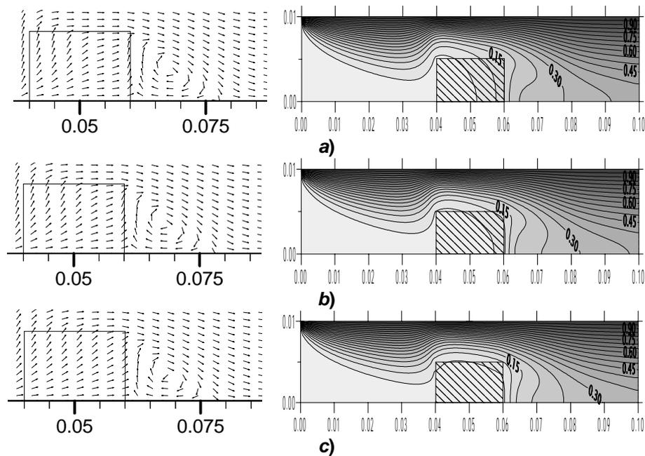
**Figure 3 – Taken from Rocamora & de Lemos, 2000b. Detailed velocity field and temperature contours for flow past a porous obstacle: a)  $K=2.0 \cdot 10^{-8} \text{m}^2$ ; b)  $K=4.0 \cdot 10^{-8} \text{m}^2$ ; c)  $K=8.0 \cdot 10^{-8} \text{m}^2$ . Refer to Fig. 2 and Table 1 for tick mark labels.**
