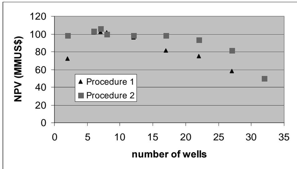
Figure 4: NPV as function of number of wells – initial well spacing of 400 m
