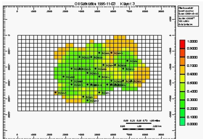
Figure 3: Residual Oil Saturation - Layer 3:
