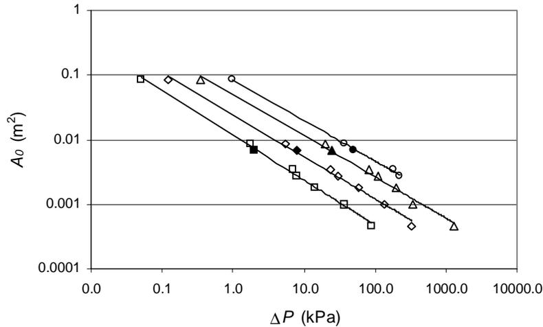
Figure 2- Estimation of number of orifices of the metallic mesh distributor.
