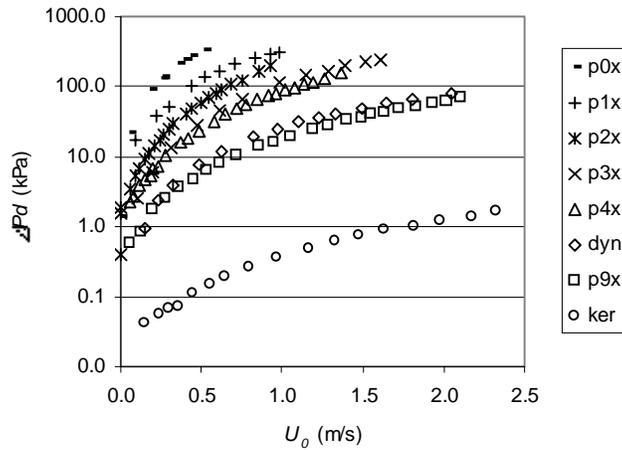
Figure 3- Pressure drop (log values) *vs* superficial velocity, different distributor plates.
