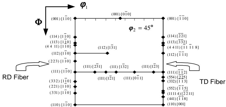
Figure 3 – Section  $\phi_2 = 45^\circ$ , Bunge notation, with the principal texture components and the RD and TD fibers (Matheus, 1999).
