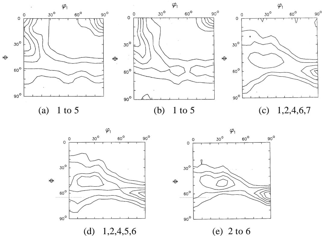
Figure 4 – CODF for 60% reduction (a) at 400°C, (b) at 600°C, (c) cold rolled and recrystallized, (d) at 400°C and recrystallized; (e) at 600°C and recrystallized. Contour values under the figures
