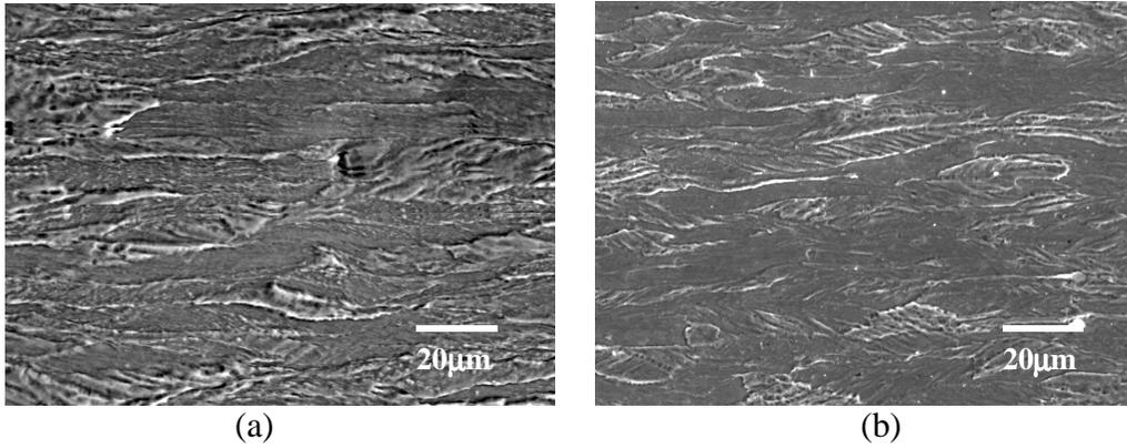
Figure 1 – Elongated grains after 60% deformation: (a) at 400°C, (b) at 600°C
