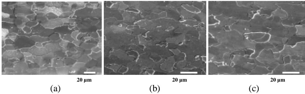
Figure 2 – 60% deformed microstructure (a) cold rolled and annealed; (b) rolled at 400°C and annealed; (c) rolled at 600°C and annealed
