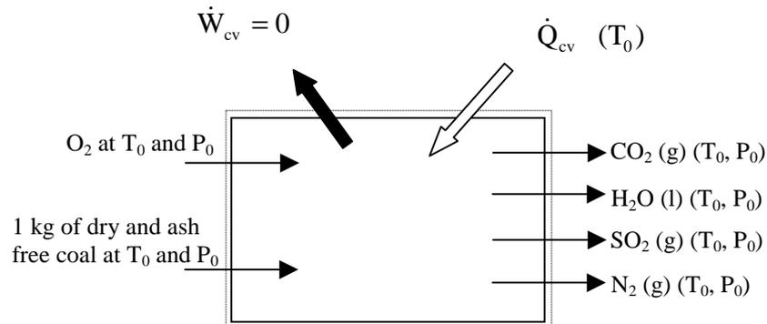
Figure 3 - Schematic view of the control volume used to evaluate the chemical exergy.
