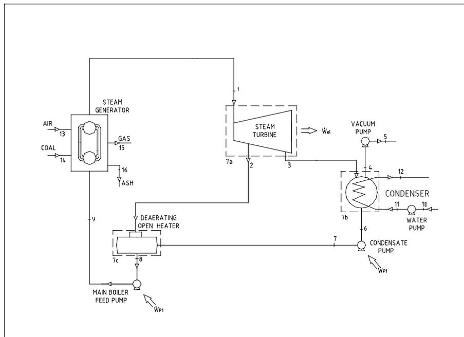
Figure 2 - Schematic view of the SIEMENS turbo-generator.
