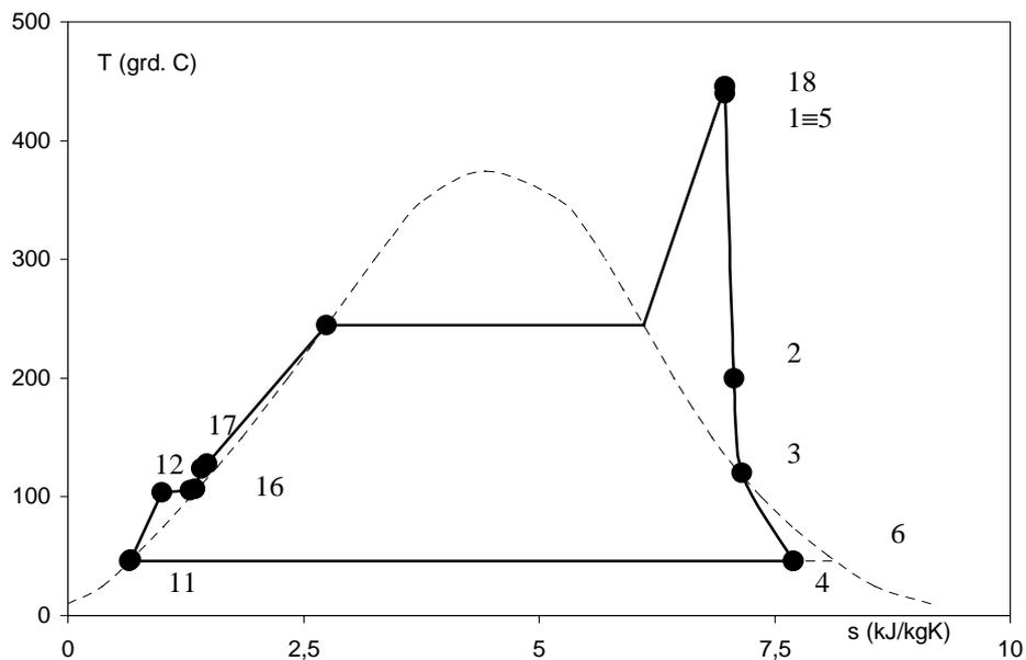
b) - T-s diagram of thermodynamic cycle A (not in scale).
