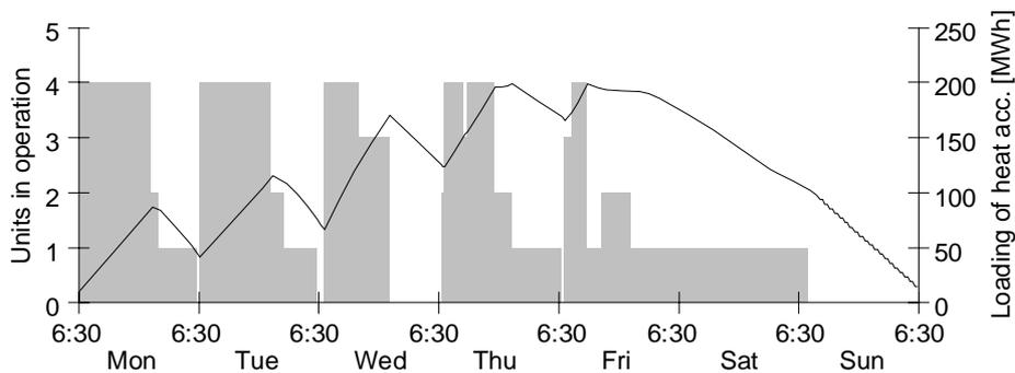
Figure 4 – Optimisation of the operation for week 22. The plant is designed with 4 gas-engines and one auxiliary boiler.
