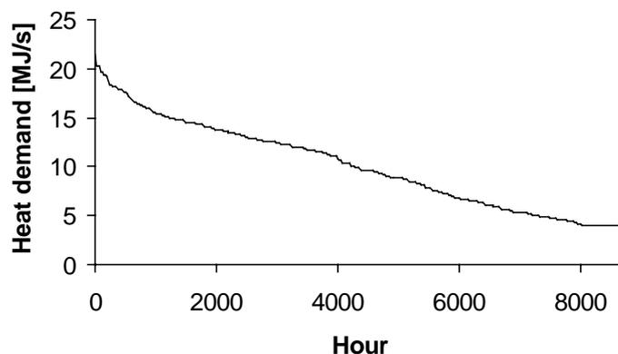
Figure 3 – Duration curve for the heat demand. It is assumed that 40% of the yearly demand is constant load.
