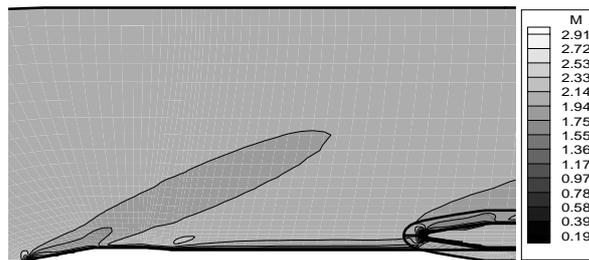
Figure 6-Mach number contours for a longitudinal plane including the central body and booster for  $M_\infty = 2$  and  $\alpha=0$  deg.
