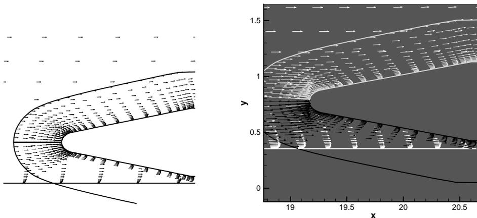
Figure 7-Velocity vector field in the overlapping region. Central body grid has: (a) 80 x 40 x 13 points; (b) 100 x 40 x 13 points.
