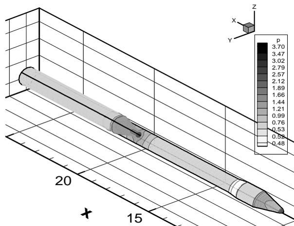
Figure 5-Pressure contours along the VLS main body and booster walls for  $M_\infty = 2$  and  $\alpha = 0$  deg.
