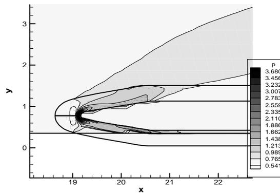
Figure 8-Pressure contours in the overlapping region for the central body grid with 100 x 40 x 13 points.
