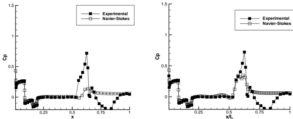
Figure 9 –Comparison of  $C_p$  between numerical and experimental results in the wall of the VLS central body for  $M_\infty = 2$  and  $\alpha = 0$  deg. Central body grid has: (a) 80 points in the  $\xi$  direction; (b) 100 points in the  $\xi$  direction.
