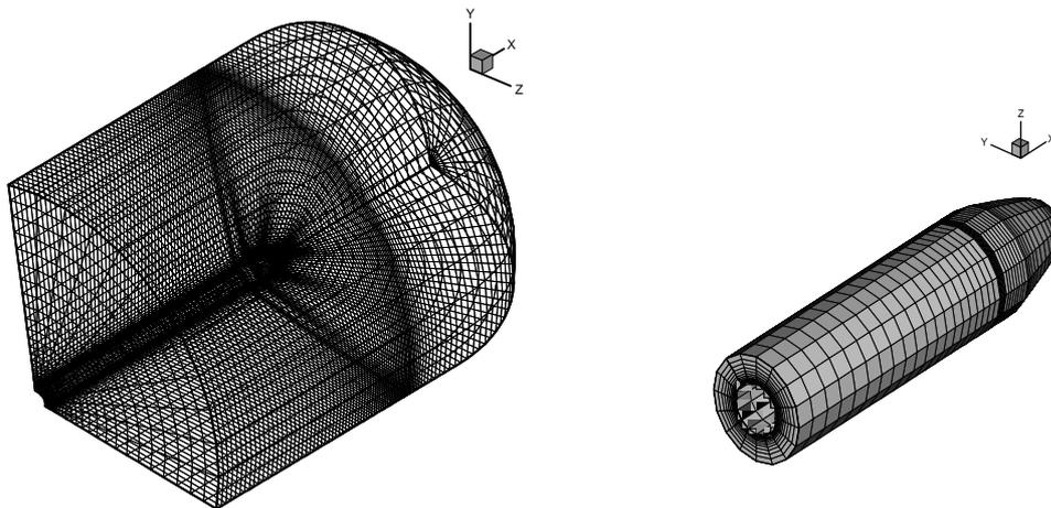
Figure 2-View of the VLS central core grid and booster grids.
