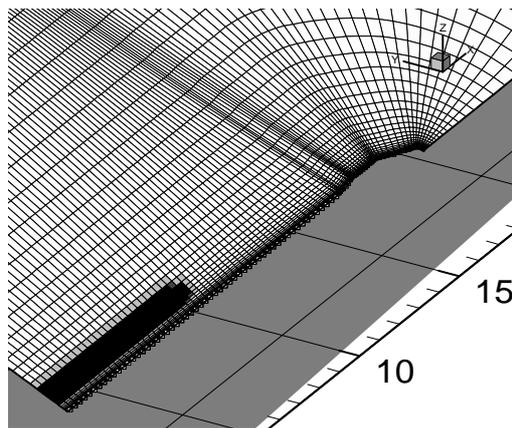
Figure 4-The VLS central body grid with the hole in one plane.
