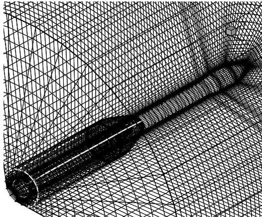
Figure 3-Overlapping region between VLS central body grid and booster grids.
