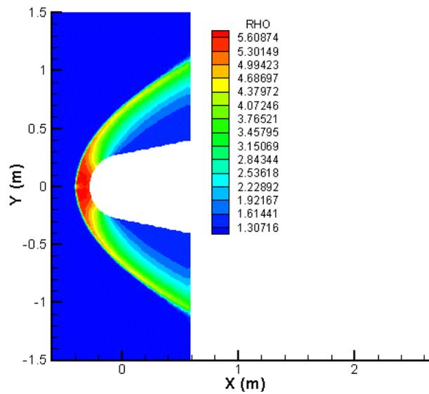
Figure 10 – Density contours obtained using 2nd-order van Leer scheme ( $M_\infty = 10$ )
