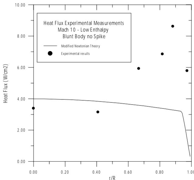
Figure 6 - Heat flux at “double Apollo disc” model.
