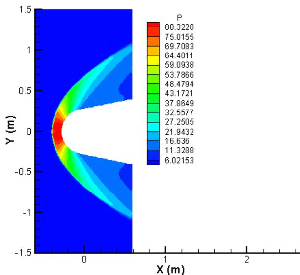
Figure 9 – Pressure contours obtained using 2nd-order van Leer scheme ( $M_\infty = 10$ )
