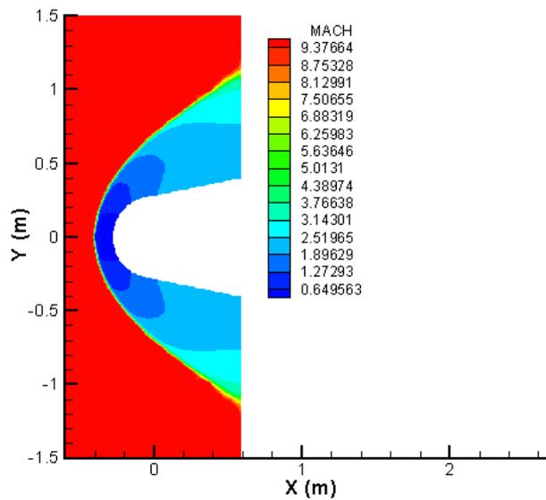
Figure 8 - Mach number contours obtained using 2nd-order van Leer scheme ( $M_\infty = 10$ )
