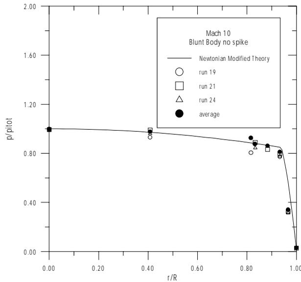
Figure 5 - Pressure ratio at “double Apollo disc” model.
