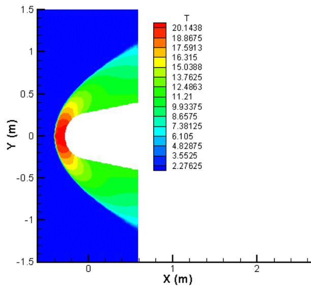
Figure 11 – Temperature contours obtained using 2nd-order van Leer scheme ( $M_\infty = 10$ )
