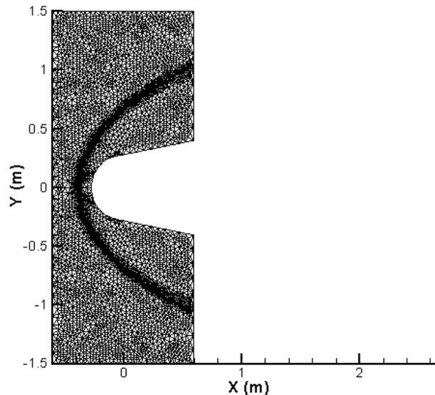
Figure 7 – Adaptive mesh obtained with one pass of refinement
