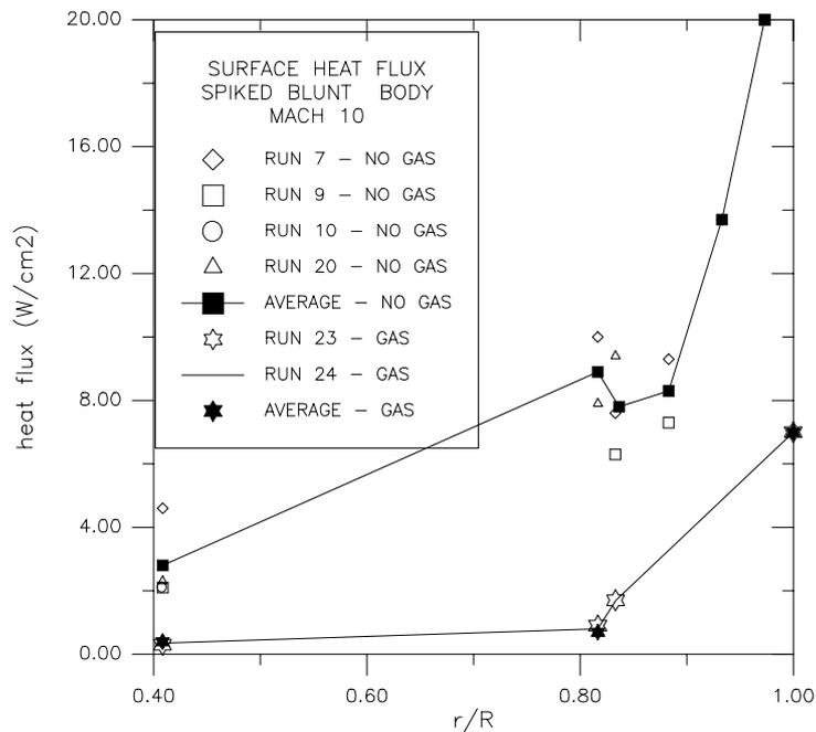
Figure 9 - Heat flux for spiked blunt body with and without cooling gas.
