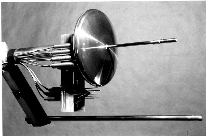
Figure 3 - “double Apollo disc” model equipped with the spiked and pressure transducers.
