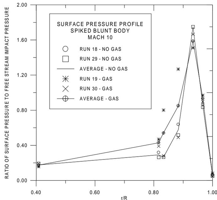
Figure 8- Pressure ratio for spiked blunt body with and without cooling gas
