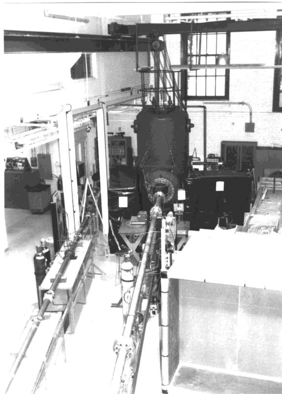
Figure 4 - RPI 24-in. diameter Hypersonic Shock Tunnel.
