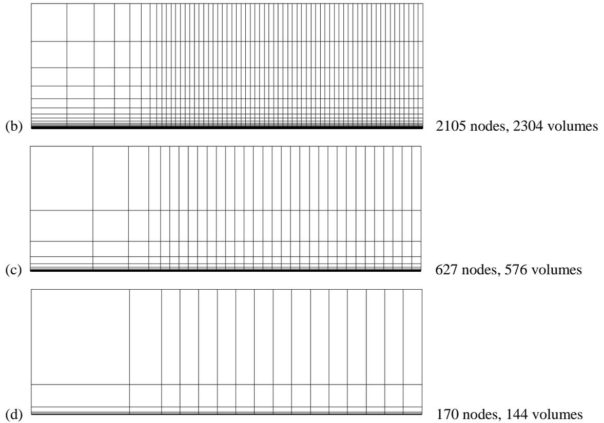
Figure 2: Fine (a) and coarse agglomerated meshes (b, c, d) used for the flat plate calculation.
