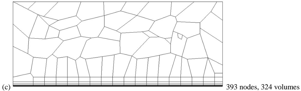
Figure 5: Hybrid meshes for a flat plate. Mesh (a) is the original mesh, while meshes (b) and (c) are coarse agglomerated meshes.
