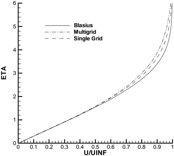
Figure 4: Comparison of the numerical results obtained with the Blasius solution for the flat plate ( $M_\infty = 0.3$  and  $Re = 1.0 \times 10^5$ ).
