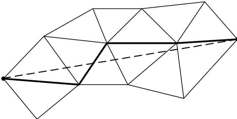
Figure 1: Mesh simplification by the node elimination procedure.
