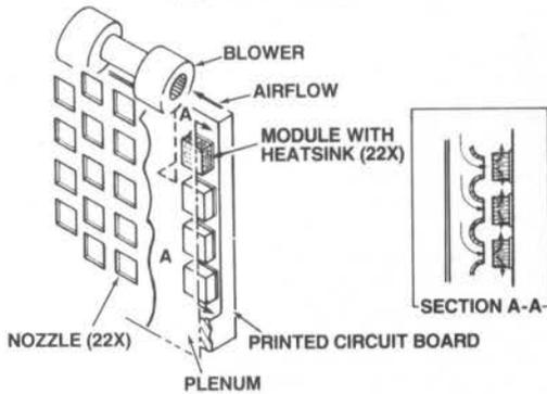
**Figure 2B: The IBM 4381 Air-Cooled Module**
