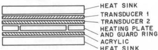
Figure 6. In line arrangement for calibration.
