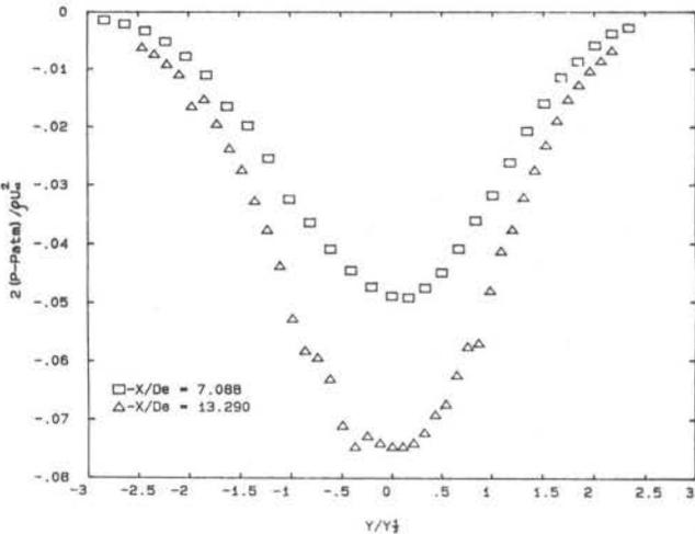
Fig. 8 Fully developed region static pressure profiles in the central X-Y plane.
