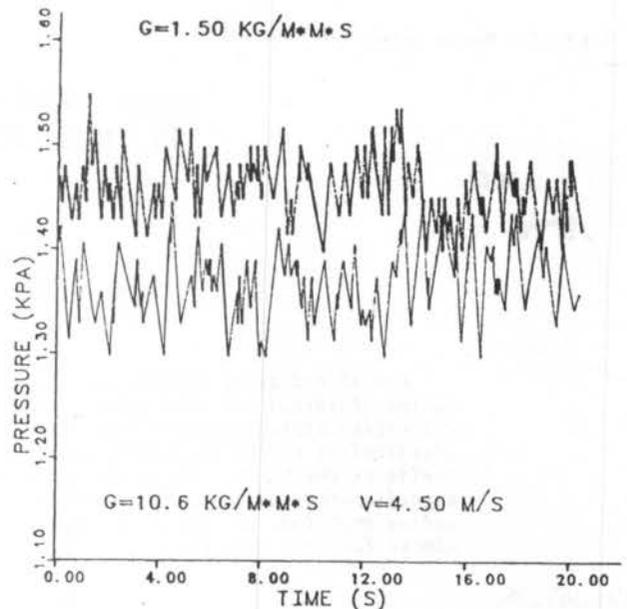
Figure 3. Typical pressure fluctuations as a function of time for different loadings.
