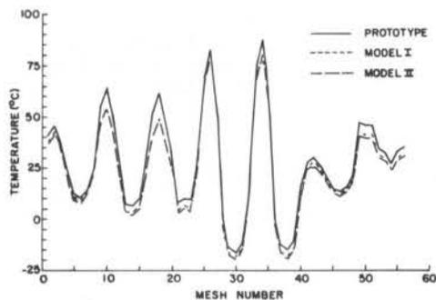
Figure 3. Temperature Distributions for Prototype and Models I and II for Steady State Conditions.
