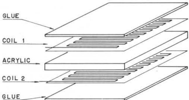
Figure 1. Exploded-view of transducer body.
