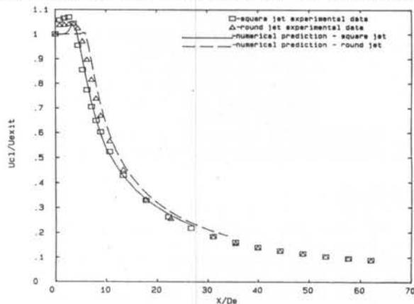
Fig. 2 Centerline mean streamwise velocity decay.
