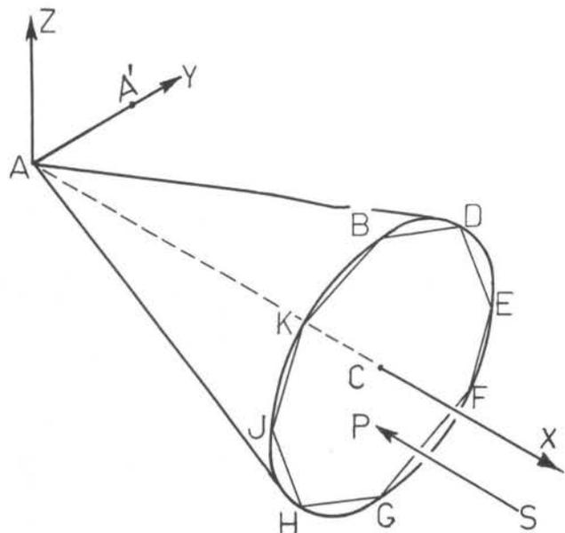
Figure 1. Conical cavity and its global frame of reference in isotropic view.
