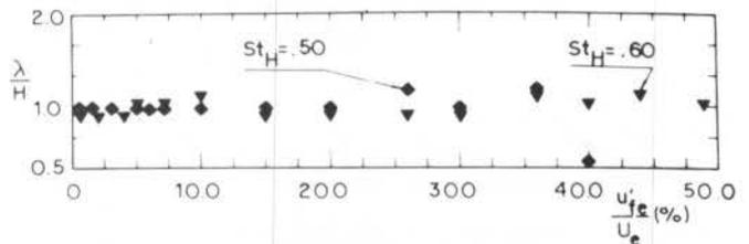
Figure 6. Distribution of  $\lambda/H$  vs  $u'_{fe}/U_e$  in the shear layer region ( $U/U_c = 0.5$ ) and  $1.0 < x/H < 2.0$ .
