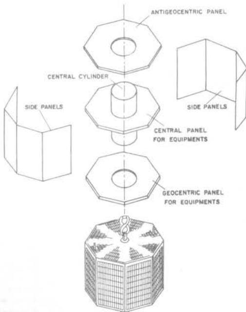
Figure 1. Schematic View of the First Brazilian Type Spacecraft
