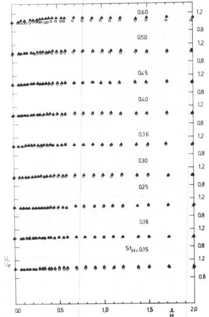
Figure 3. Axial variation of the mean velocity distribution along the jet center line. o, unforced;  $\blacktriangle$ , forced data ( $u'_{fe}/U_e = 7.2\%$ )
