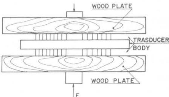
Figure 3. Mechanical device for transducer gluing.
