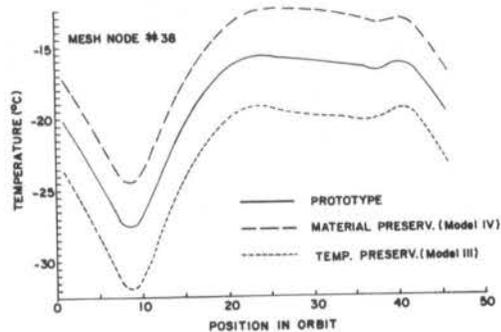
Figure 5. Transient Temperature Behavior of Prototype and Models III and IV (Mesh Node # 38)
