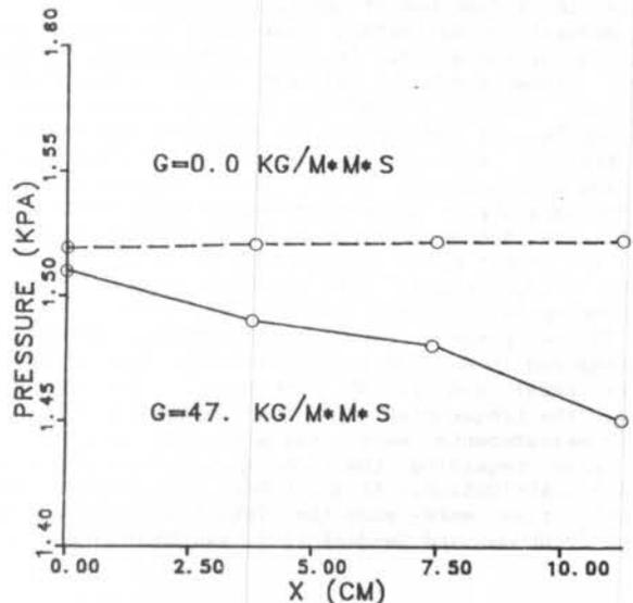
Figure 4. Variation of the mean pressure in the radial direction for different loadings.
