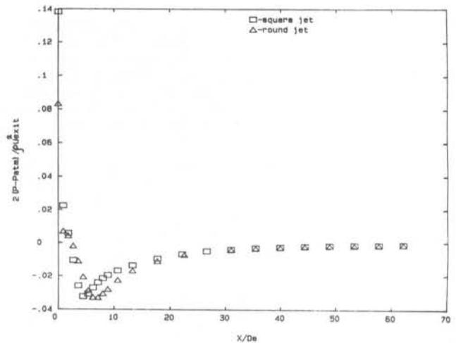
Fig. 6 Centerline static pressure distributions.
