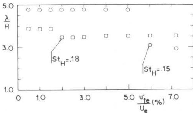
Figure 5. Distribution of  $\lambda/H$  vs  $u'_{fe}/U_e$  in the shear layer region ( $U/U_c = 0.5$ ) and  $1.0 < x/H < 2.0$ .
