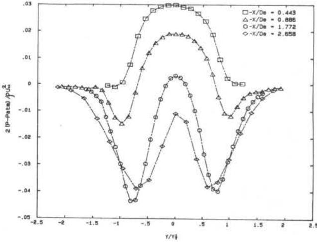
Fig. 7 Initial region static pressure profiles in the central X-Y plane.
