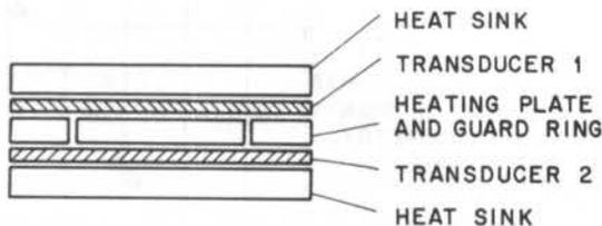
Figure 7. Symmetric arrangement for calibration.
