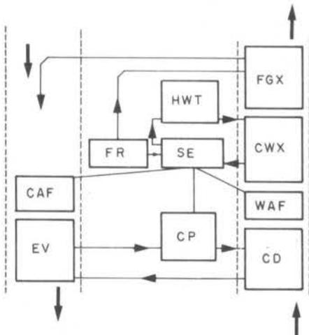
Figure 1. Diagram of a Stirling engine driven heat pump [17]
