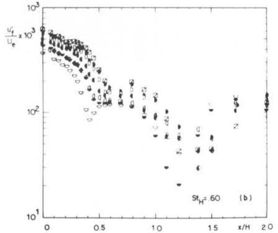
Figure 2.  $u'_f$  vs  $x/H$  measured at the shear layer region ( $U/U_c = 0.5$ )
