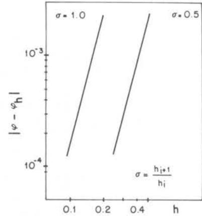
Fig. 2 Error for 2-D Poisson Equation. Effect of Non-uniform mesh size.
