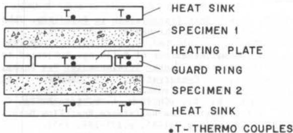
Figure 5. Guarded Hot Plate Apparatus.
