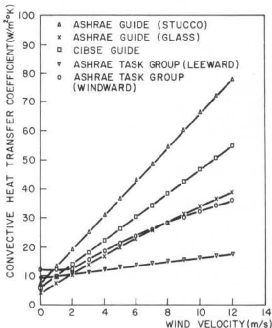
Figure 2. Comparison between guide recommendations for the convective heat transfer coefficient on building's facades.
