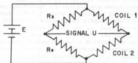
Figure 4. Signal generation using a Wheatstone Bridge.
