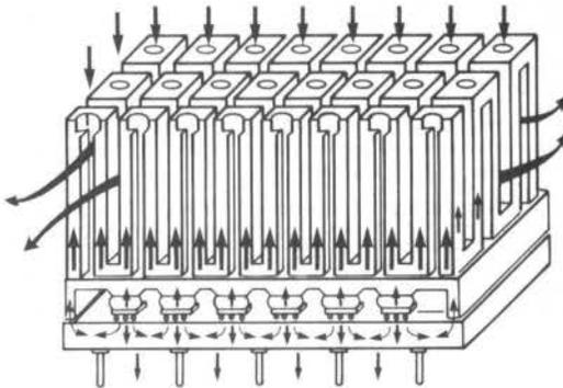
Based on information provided in [10], it appears that 55% of the heat released by the chips conducts down into the MLC substrate and 45% up through the thermal paste to the cap. However, more than half of the heat flowing into the MLC conducts back up through the solder seal to the cap. Thus, in total, nearly 75% of the dissipated heat exits the module via the fin array and the remainder is removed at the exposed surfaces of the board.
