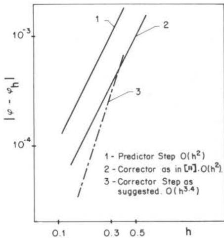
Fig. 3 Error for 2-D Poisson Equation. Effect of deferred corrections.
