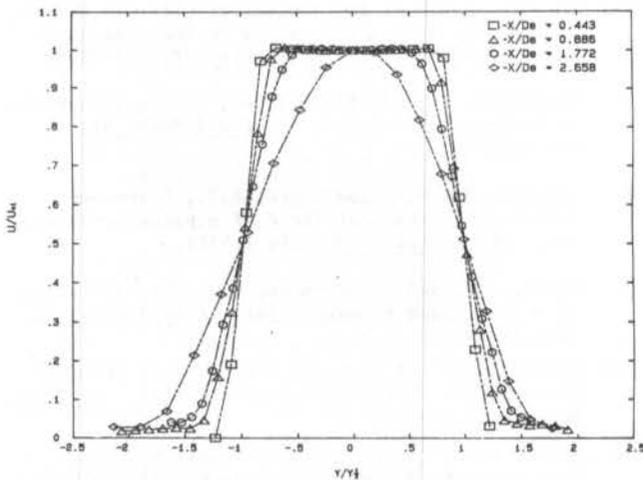
Fig. 3 Initial region mean streamwise velocity profiles in the central X-Y plane.
