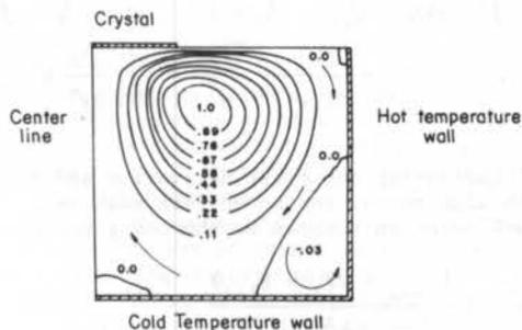
Fig. 5 Stream Function Contours for Bottom Cooled Crystal Growth With Aspect Ratio = 1,0 Rayleigh Number =  $5 \times 10^4$  Reynolds Number = 25.0 and  $\theta_b = 0$  Maximum Stream Function is 39.59 at (0.44, 0.25)
