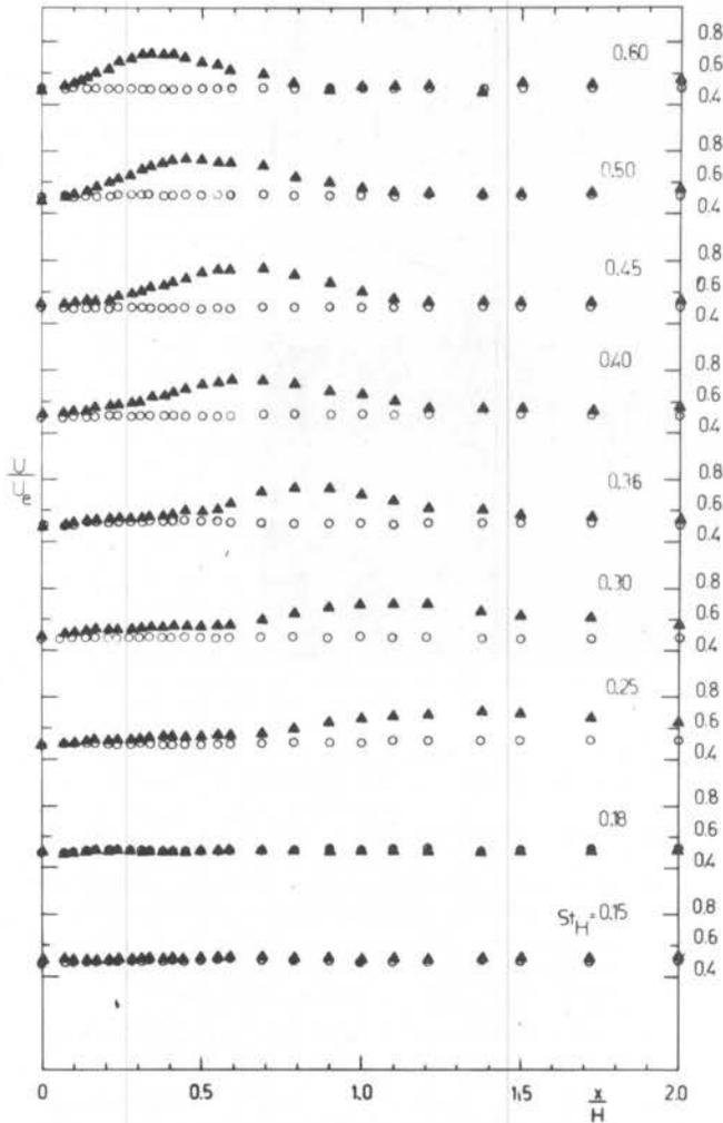
Figure 5. Measurements of the mean velocity in the region (at  $U/U_c = 0.5$ ). o, unforced;  $\blacktriangle$ , forced data ( $u_{fe}^1/U_e = 7.2\%$ )
