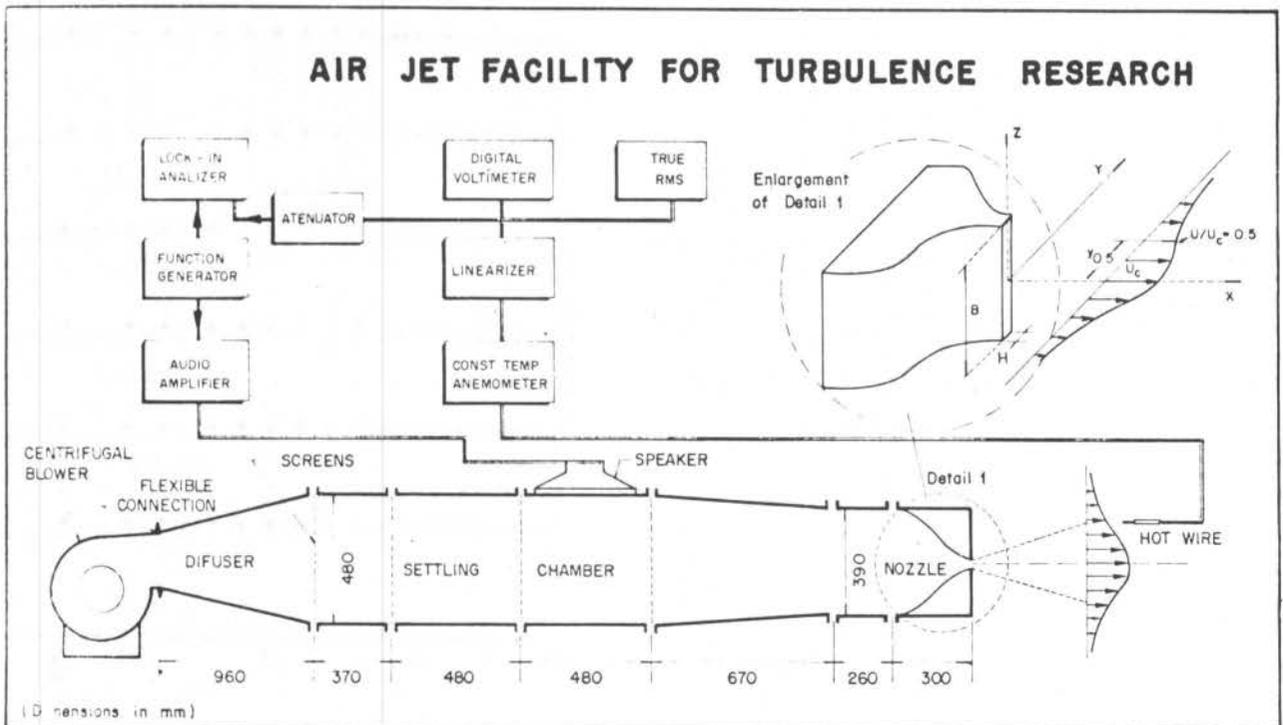
Figure 1. Schematic of the plane jet flow facility and data acquisition system
