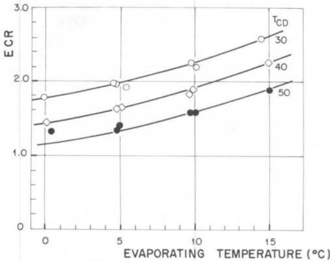
Figure 2. Variation of the energy conversion ratio of an engine driven heat pump
