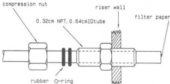
Figure 2. Static pressure radial probe.
