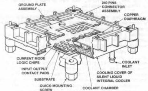
Unfortunately, while Honeywell was one of the first companies to develop water cooling for mainframe computers, little additional information is available in the open literature on the thermal performance of the SLIC. For an assumed water inlet temperature of 24°C, as well as a peak allowable chip temperature of 70°C and a maximum chip dissipation of .75 W, the overall thermal resistance of the SLIC can be calculated to equal approximately 60 K/W.
