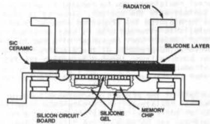
The Hitaceram 101 SiC RAM module contains 6, 1-Watt, ECL chips, each 1.9 x 4 mm and providing 1 kbit of memory, solder-bumped to a silicon substrate which is, in turn, gold/tin eutectic bonded to the SiC. Both the Aluminum fin structure and the lid are attached to the module with a layer of silicone rubber (with filler), approximately 50 micron thick. The chips are encapsulated in silicone gel for protection from humidity and from alpha particles emanating from the solder.
