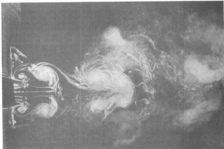
Figure 7(a,b). Smoke-wire flow visualization experiments ( $Re = 6750$ ;  $St_H = 0.60$ )
