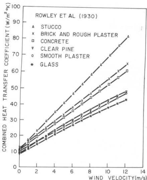
Figura 1. Surface heat transfer as a function of wind speed.
