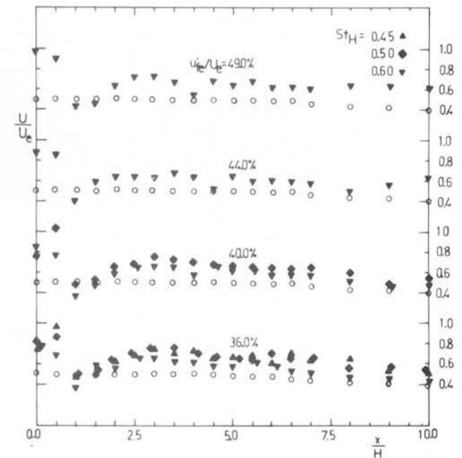
Figure 6. Measurements of the mean velocity in the region (at  $U/U_c = 0.5$ ). o, unforced;  $\blacktriangle$ , forced data ( $u_{fe}^1/U_e = 40\%$ )
