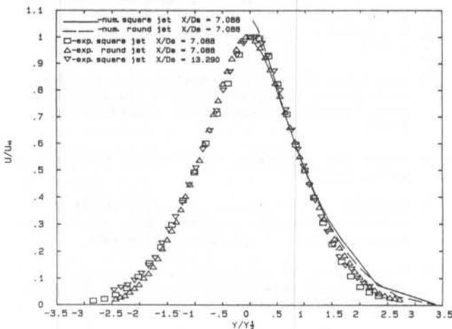
Fig. 4 Fully developed region mean streamwise velocity profiles in the central X-Y plane.
