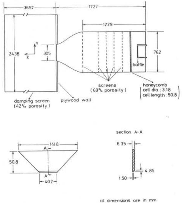
Fig. 1 Experimental set-up: (a) plan view section through the settling chamber, contraction and screen cage, (b) square slot detail.
