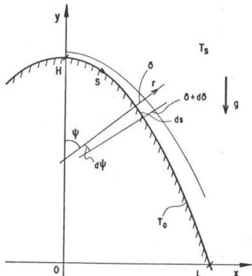
FIGURE 1 - Film condensation on Curved surfaces
