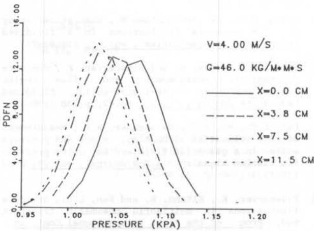
Figure 5. The probability density function distribution of the radial static pressure fluctuations.
