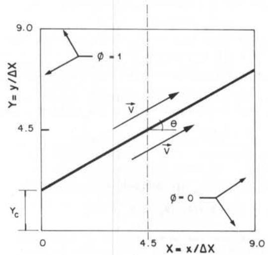
Figure 4. Step-Profile in a Uniform Flow at an Angle
