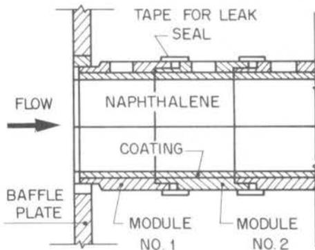
Figure 2. The test section
