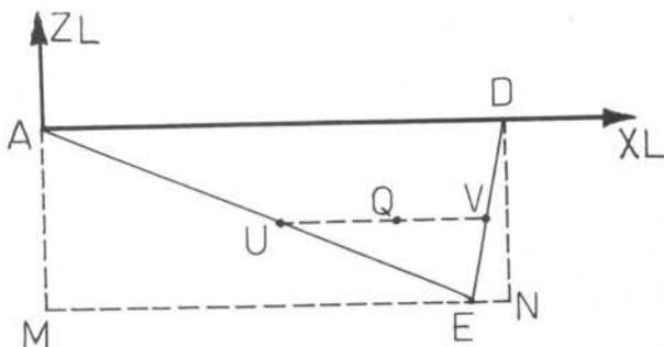
Figure 3. Element ADE and its envelope AMEND in XL-ZL plane of its local frame.
