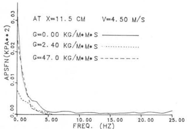
Figure 8. The power spectrum functions of the pressure signal as a function of the frequency.
