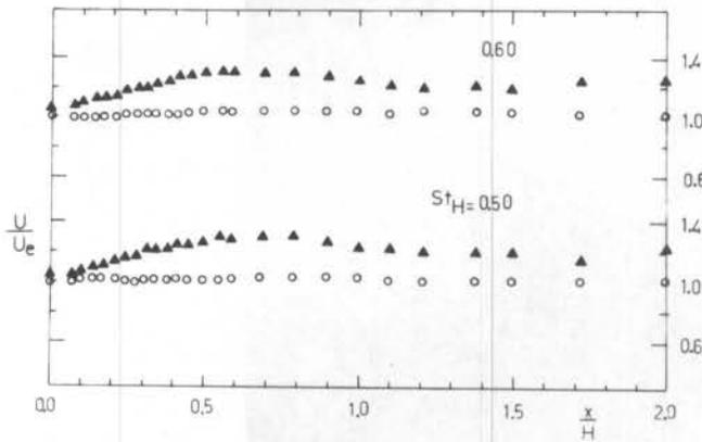
Figure 4. Axial variation of the mean velocity distribution along the jet center line. o, unforced;  $\blacktriangle$ , forced data ( $u_{fe}^1/U_e = 40\%$ )
