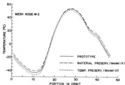
Figure 4. Transient Temperature Behavior of Prototype and Models III and IV (Mesh Node # 2)
