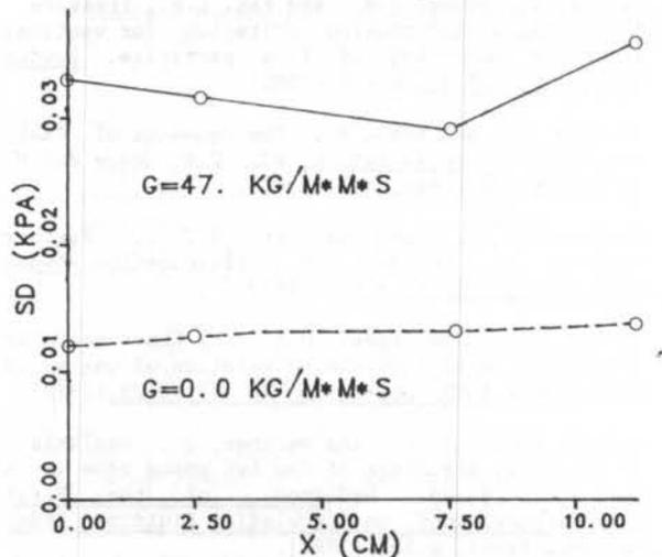
Figure 6. Variation of the standard deviation of the pressure fluctuations with the solids mass flow rate.
