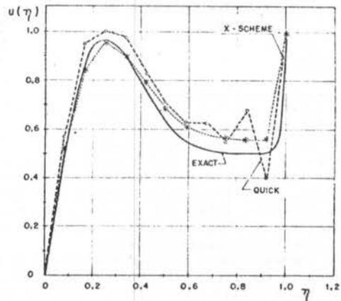
Figure 1. Velocity profile comparing QUICK (divergent formulation) and the proposed scheme (convective formulation).  $\text{Re}_c = 10^3$
