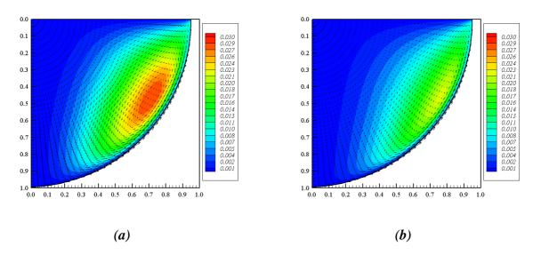
**Figure 3.** Stream-function and velocity vectors for t = 1, (a)  $Re_o = 10$  and (b)  $Re_o = 100$  —  $121 \times 121$  grid,  $\tau = 2.5$ ,  $u_{\theta,s} = sin(2\theta)$ ,  $u_{r,max} = 10^{-5}$
