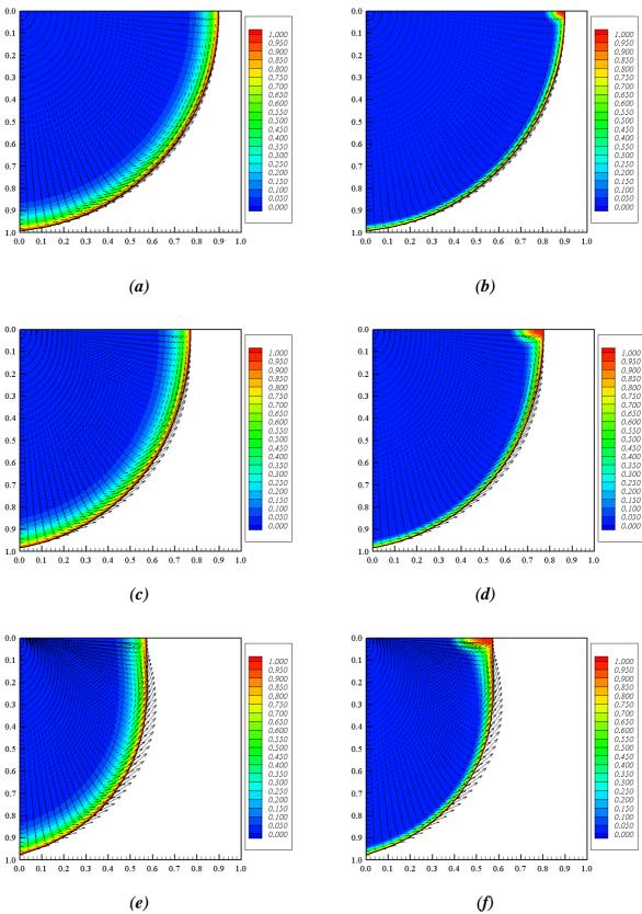
**Figure 4.** Temperature field and velocity vectors for  $Re_o = 10 - t = 2$  (*a*), t = 4 (*c*), t = 6 (*e*) – and  $Re_o = 100 - t = 2$  (*b*), t = 4 (*d*), t = 6 (*f*) –  $-121 \times 121$  Grid Points,  $u_{\theta,s} = \sin(2\theta), u_r = 10^{-5}$ .
