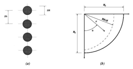
**Figure 1**. Sketch of (a) the center portion of an infinite stream of droplets and (b) of the physical domain with principal dimensions and deformed droplet surface.
