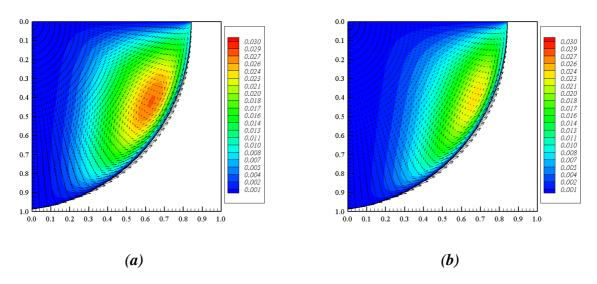
**Figure 4.** Stream-function and velocity vectors for t = 3, (a)  $Re_o = 10$  and (b)  $Re_o = 100$  —  $121 \times 121$  grid,  $\tau = 2.5$ ,  $u_{\theta,s} = sin(2\theta)$ ,  $u_r = 10^{-5}$
