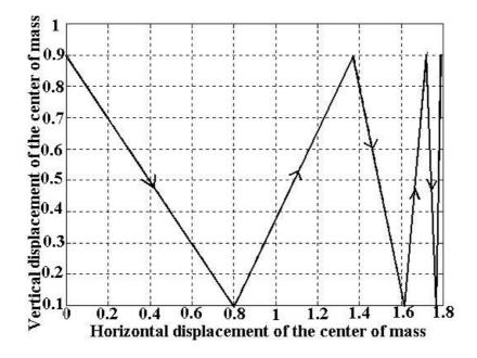
Figure 5. The C-S model using  $e_{mC} = e_{mE} = -1$ ,  $e_t = 0$  and v = 0. Units (m).
