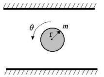
Figure 4. Collision of a ball with two barriers.
