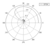
Figure 4. Case II:  $\varepsilon = 0.5$ , W = 33.6 Kg, c = 1.016e-4 m,  $r_b = 6.477e-2$  m, L = 1.143e-2m,  $F_u = 100$  N,  $V_b = 5000$  rpm,  $\eta = 2.622e-3$  Ns/m<sup>2</sup>.
