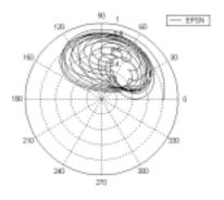
Figure 7. Case V:  $\varepsilon = 0.8$ , W = 33.6 Kg, c = 2.54e-4 m,  $r_b = 2.54e-2$  m, L = 5.08e-2 m,  $F_u = 300$  N,  $V_b = 5000$  rpm,  $\eta = 8.276e-3$  Ns/m<sup>2</sup>.
