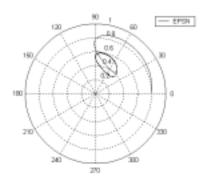
Figure 8. Case VI:  $\varepsilon = 0.8$ , W = 33.6 Kg, c = 2.54e-4 m,  $r_b = 2.54e-2$  m, L = 5.08e-2 m,  $F_u = 100$  N,  $V_b = 2000$  rpm,  $\eta = 2.53e-2$  Ns/m<sup>2</sup>.
