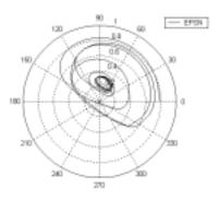
Figure 9. Case VII:  $\varepsilon = 0.8$ , W = 33.6 Kg, c = 2.54e-4 m,  $r_b = 2.54e-2$  m, L = 5.08e-2 m,  $F_u = 100$  N,  $V_b = 4000$  rpm,  $\eta = 2.53e-2$  Ns/m<sup>2</sup>.
