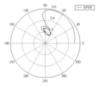
Figure 2. Case I:  $\varepsilon = 0.5$ , W = 33.6 Kg, c = 1.016e-4 m,  $r_b = 6.477e-2$  m, L = 1.143e-2m,  $F_u = 100$  N,  $V_b = 2000$  rpm,  $\eta = 2.622e-3$  Ns/m<sup>2</sup>.
