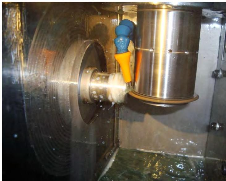
Figure 3. Ultraprecision grinding process of the Tungsten Carbide Cobalt (WC-Co)
