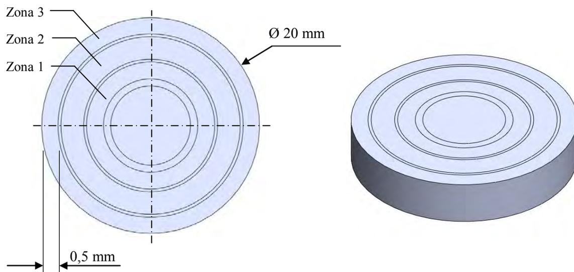
Figure 2. Illustration of the three zones of grinding in tungsten carbide samples
