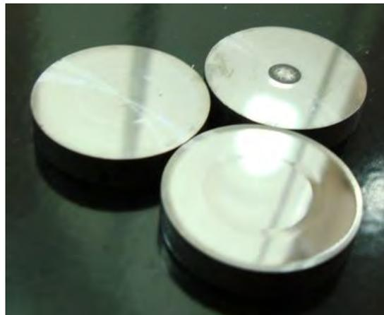
Figure 6. Tungsten carbide surfaces generated by Ultraprecision Grinding.
