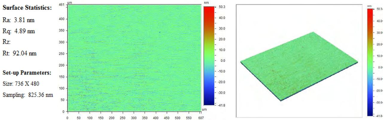
Figure 4. Three-dimensional WYKO interference image revealing the surface roughness of the ground 88%WC.
