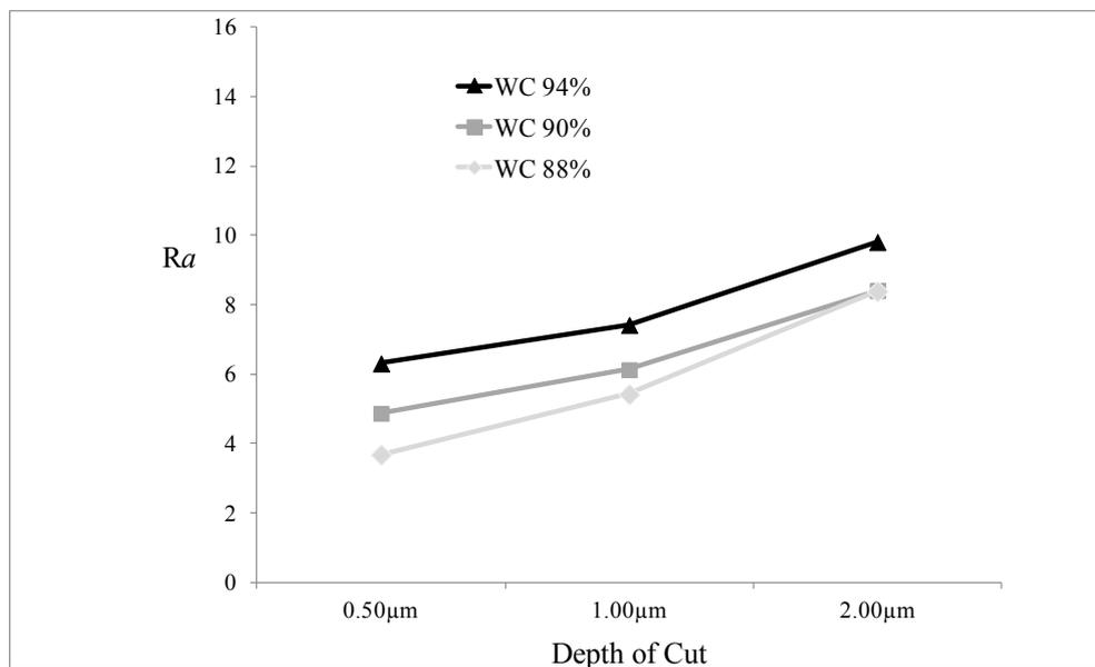
Figure 5. Surface roughness (Ra) versus microstructure of carbide materials and depth of cut.
