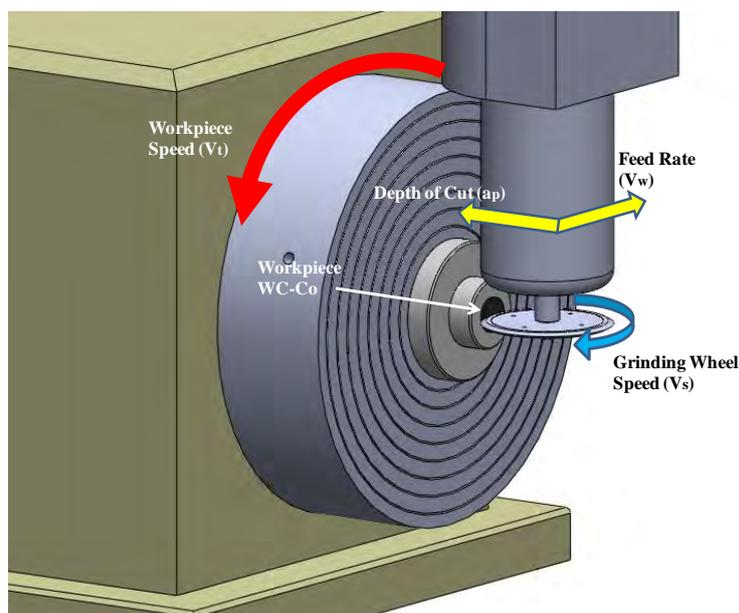
Figure 1. Grinding process kinematics of the Tungsten Carbide Cobalt (WC-Co)
